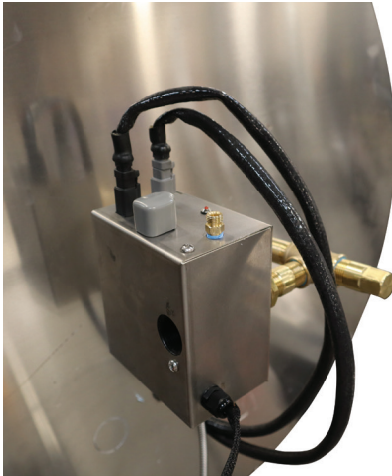
Photo 11: Electronic Connections from the Pilot to Valve
