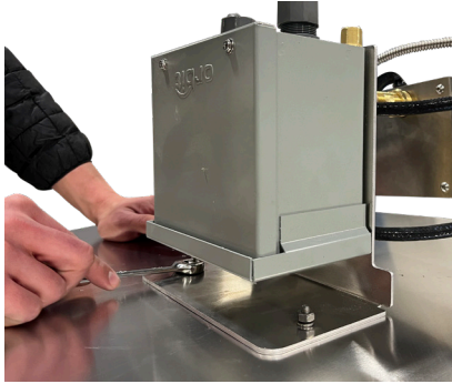
Photo 13: Mounting the Transformer to the Plate
