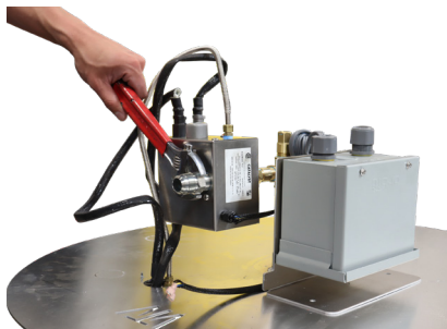
Photo 20: Connecting the Flared Fitting to the Platinum Valve
