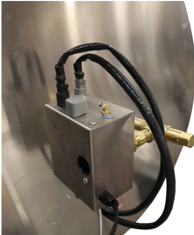
Photo 11: Electronic Connections from the Pilot to Valve
