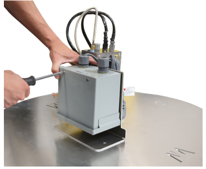
Photo 14: Removing the Front Panel
