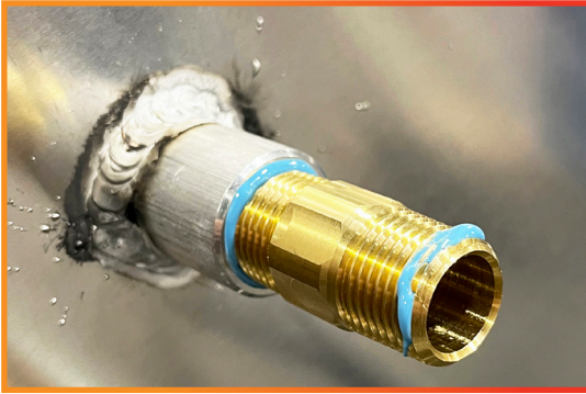
Figure 16: Attaching the 1/2" x 2" Nipple to the Plate Coupling
