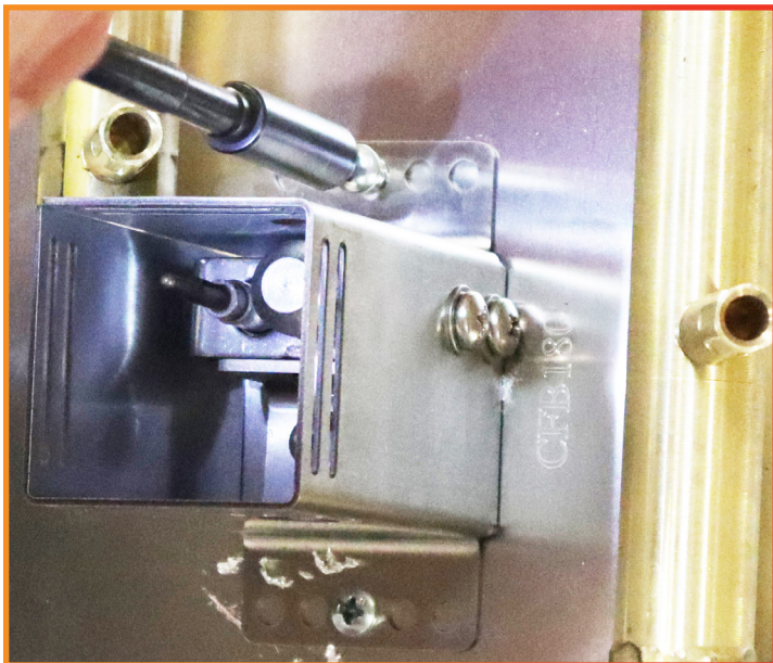
Figure 5: Securing the Pilot to the Plate/Pan
