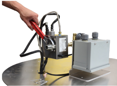
Figure 20: Connecting the Flared Fitting to the Platinum Valve
