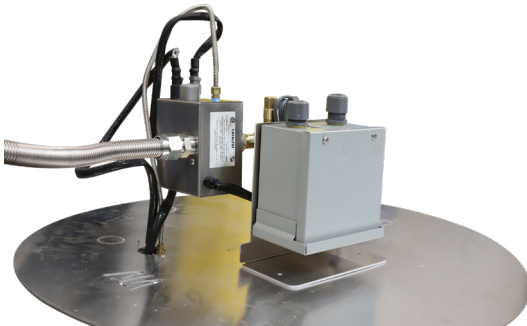
Figure 21: Attaching the Flex Line
