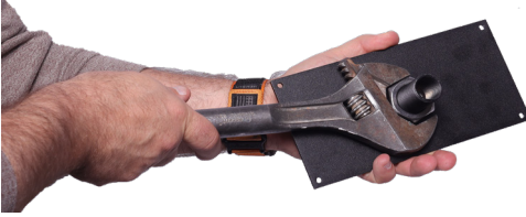
Figure 3: Attaching the nut to the Escutcheon Plate
