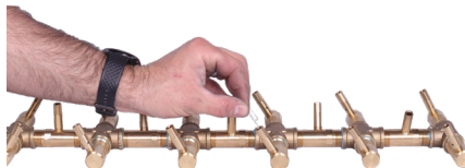
Figure 8: Cleaning the Jets
