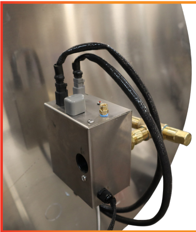
Figure 11: Electronic Connections from the Pilot to Valve
