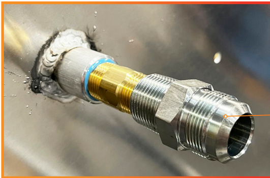
Figure 17: Attaching the Male Flare Hose Adapter
