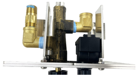
Photo 8b: Applying Joint Compound
