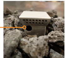
Example of proper media height on pilot assembly.
