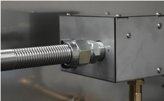
Photo 21: Attaching the Flex Line
